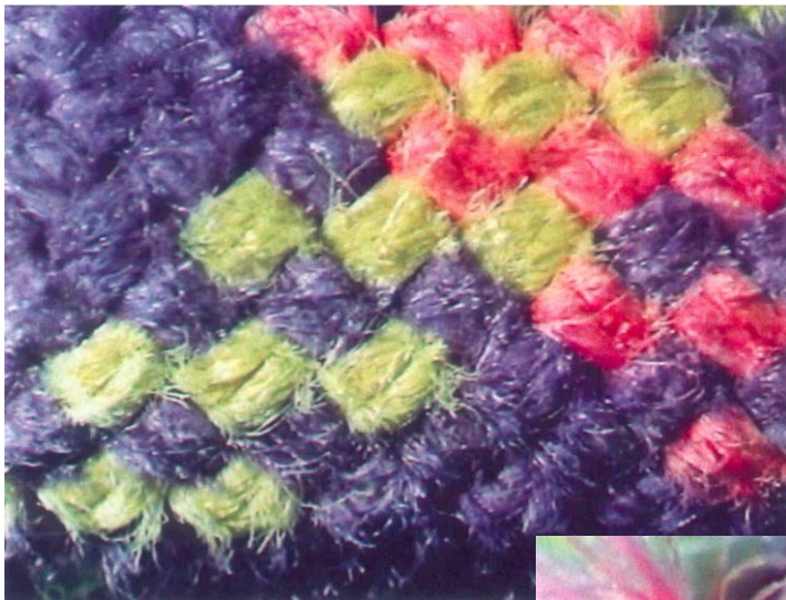
Photo 1A: Abrasion of sheath
