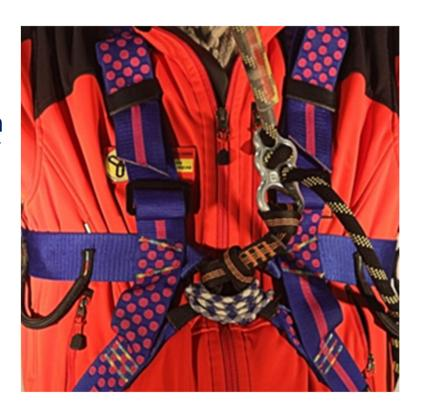
It is in any case recommended to close the harness with an additional cordellette, so that a safe anchor point is prepared for possible rescue or other manoeuvres
