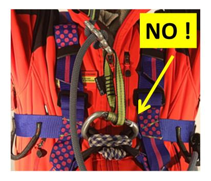
THE CARABINER COULD ACCIDENTALLY ROTATE, AND THEREFORE BE SOLICITED ALONG ITS MINOR AXIS (IN ITS WEAKEST CONFIGURATION) DURING THE FALL.
