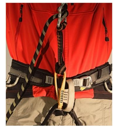
Concerning the choice of the tape loop, it is advisable to use a Nylon tape with a proper dimension, e.g. with a section of 15 mm.
