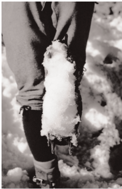
Fig. 1: Typical balling up
