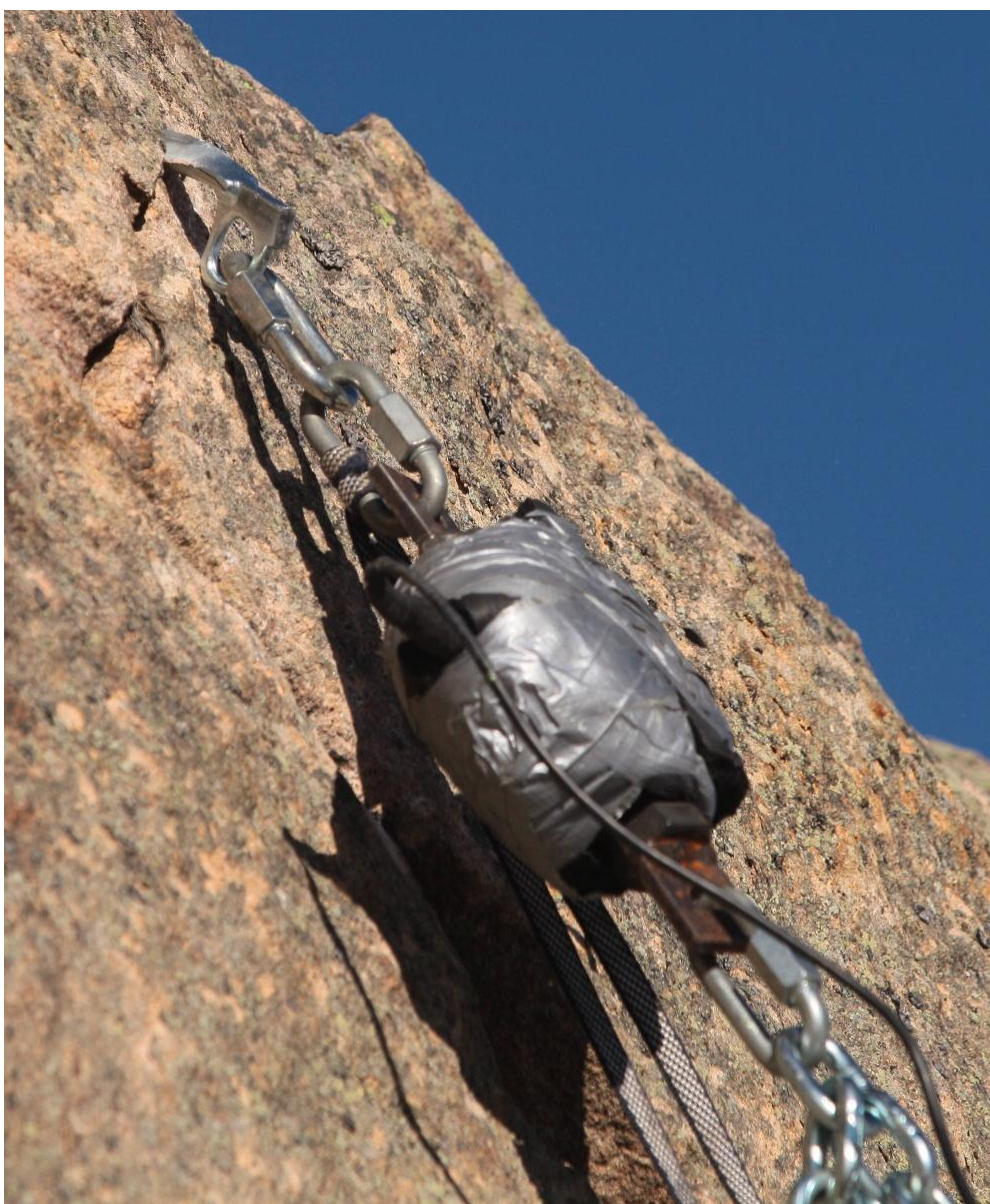
Fig.2 A picture of a test just a step before the abrupt pop out. For pitons it is evident a permanent deformation of the devices
