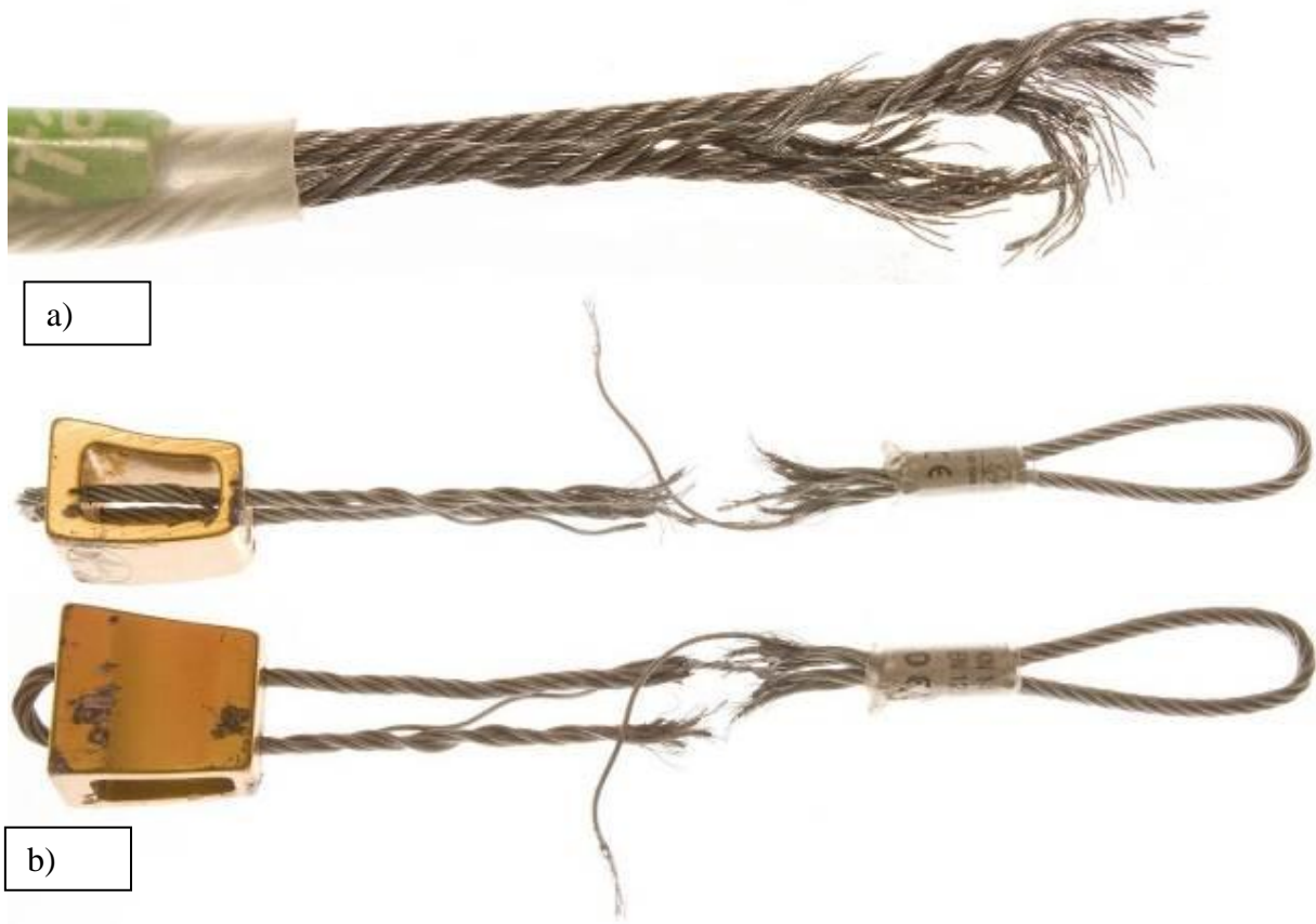
Fig.6 “Post mortem” analysis, a) failure in the wire at the loop interfacing body b) failure along the wire
