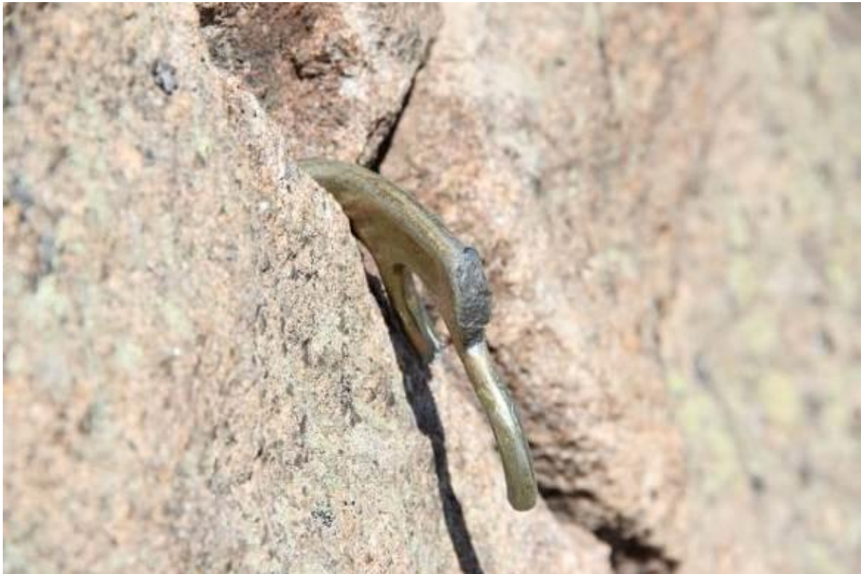
Fig.3 A picture of a failure in the piton lug after the test
