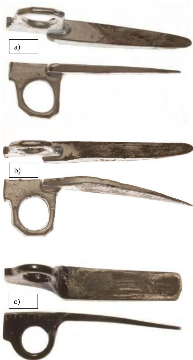
Fig.4 “Post mortem” analysis, a) soft metal piton - low residual deformation, b) soft-metal piton – medium residual deformation c) hard steel – low residual deformation
